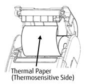
2. Please put out the edge of the paper and close the paper cover. Push two point of the paper cover firmly when closing.
