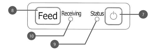
**Power Switch** : To turn the power supply ON or OFF.
