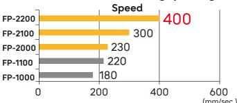
400mm/s is the Max. printing speed of FP-2200 with excellent printing quality in POS thermal printers in the world.
