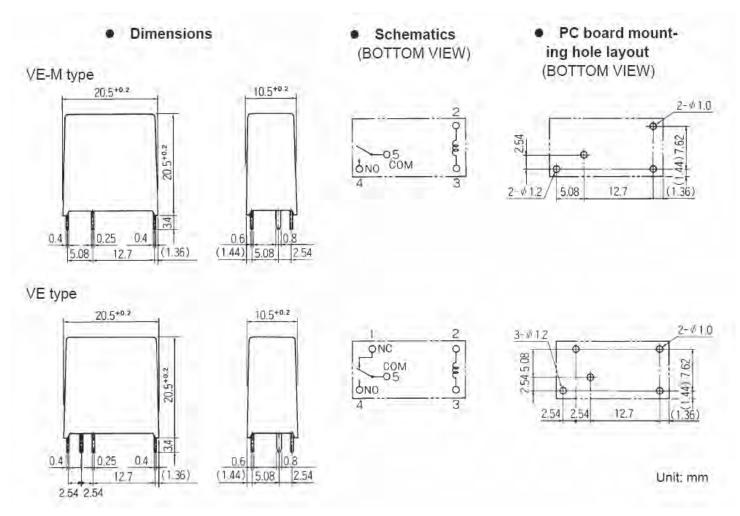
Note: This datasheet provide only + tolerance for outer dimensions.
