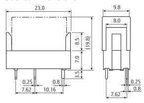
PC Board Mouting Hole Layout (BOTTOM VIEW)
