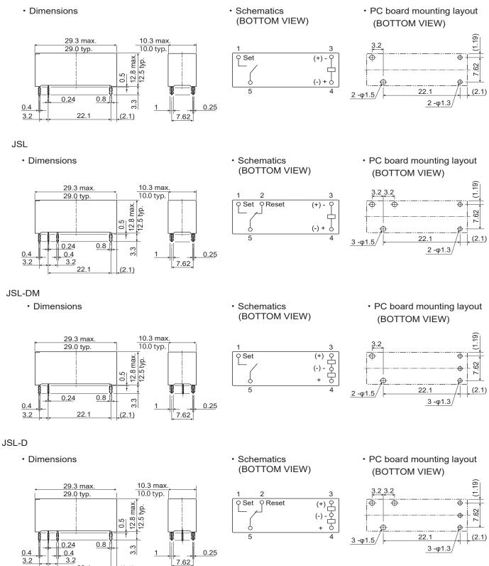
\* Dimensions of the terminals do not include thickness of pre-soldering.
