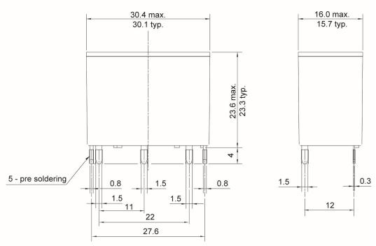
Dimensions of the terminals do not include thickness of pre-solder.
