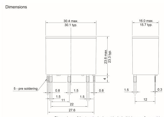
Dimensions of the terminals do not include thickness of pre-solder.
