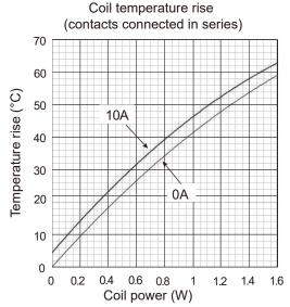
Note: When each contact is used independently, above graph shall be read; same voltage is applied on 2 coils, coil power is sum of 2 coils, applied current 10A is 10A apply on each contact set.
