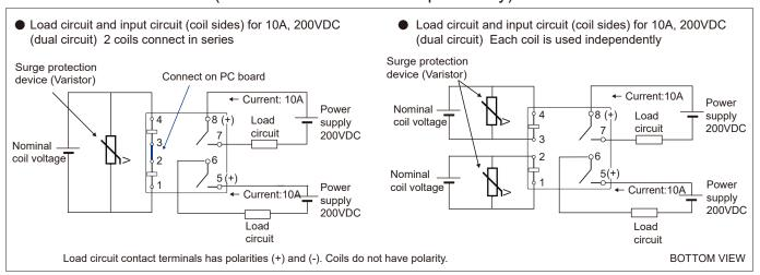
Note 1: In case 2 coils are connected in series, connect coil terminal #2 to #3 on PCB circuit. In case 2 coils are connected in parallel, connect coil terminal #1 to #3 and connect coil terminal #2 to #4 on PCB. Regarding terminal number, refer to schematics data.
