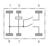
PC Board Mouting Hole Layout (BOTTOM VIEW)
