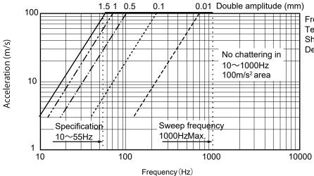
Frequency : 10 to 1000Hz Test conditions: Coil energized(12VDC) and de-energized Shock direction: see diagram below Detection level: chatter >1ms
