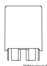
COM terminal: 2.5 x 0.32t Coil terminal: 1.0 x 0.3t N.O. terminal: 2.5 x 0.5t N.C. terminal: 1.3 x 0.4t
