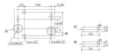
Tolerance of PC board mounting hole layout : ±0.1 unless otherwise specified.
