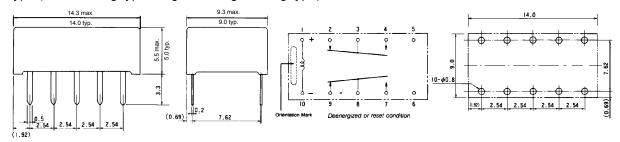
AL-D type (Double winding latching type)
